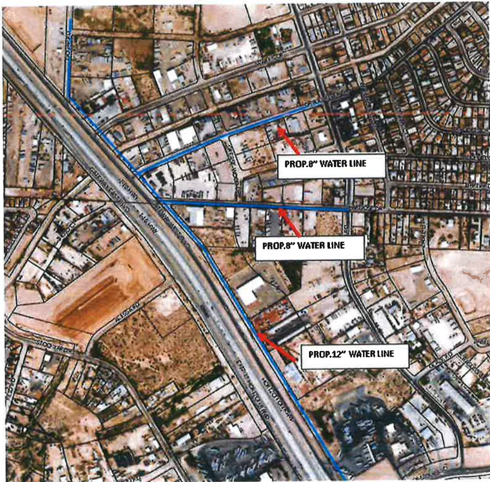
Figure 2 - Gateway West Blvd Water (Site Plan)
